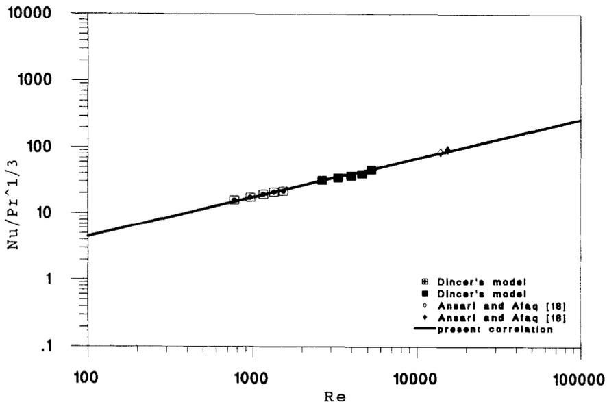
FIG. 4. The diagram of  $Nu/Pr^{1/3}$  vs Reynolds number for cylindrical products.
