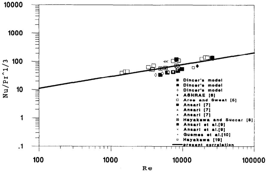
FIG. 3. The diagram of  $Nu/Pr^{1/3}$  vs Reynolds number for spherical products.
